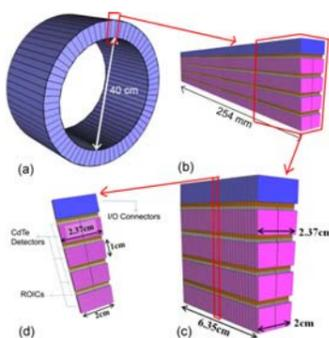
Figure 1-a shows the full VIP scanner. 1-b, is a one sector of the scanner and 60 of these sectors are needed to form the full scanner. In 1-c, one can see section of the sector 1-b. 1-d is the VIP kernel detector module for the VIP scanner and it as 800 channels with 800 voxels, each has a volume of  $1 \times 1 \times 2 \text{ mm}^3$  of CdTe
